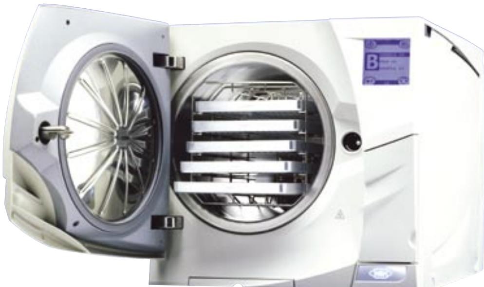
All Sendoline instruments are non-hollow, non-porous loads and can be sterilized in a normal gravity-process sterilizer at 134 degrees Celsius, at a minimum holding time of 3 minutes.
